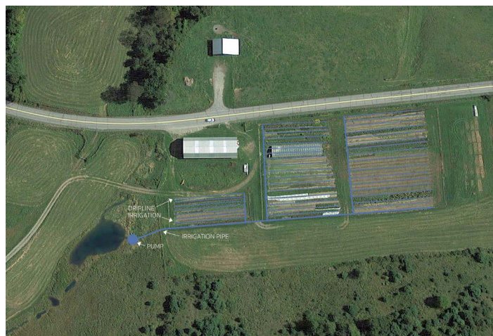
Diagram of pump and irrigation system installed.
